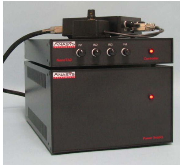
The nano-TA2 electronics comprising the power supply, TMA controller and CAL box.
