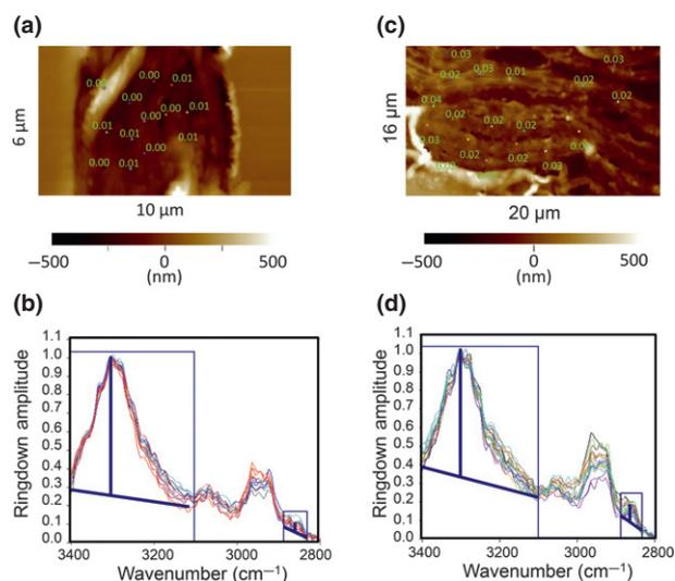
**Figure 1.** Contact-mode AFM height image (a) and 13 AFM-IR spectra (b) of a delipidized SC cross-section. Contact-mode AFM height image (c) and 18 AFM-IR spectra (d) of a normal SC cross-section. The coloured marker locations (each representing a  $20 \times 100$  nm area of the sample) on the AFM images (a, c) are labelled with the ratio of the baseline-corrected band intensities of the 2856 and 3290/cm peaks corresponding to the spectrum of the same colour.
